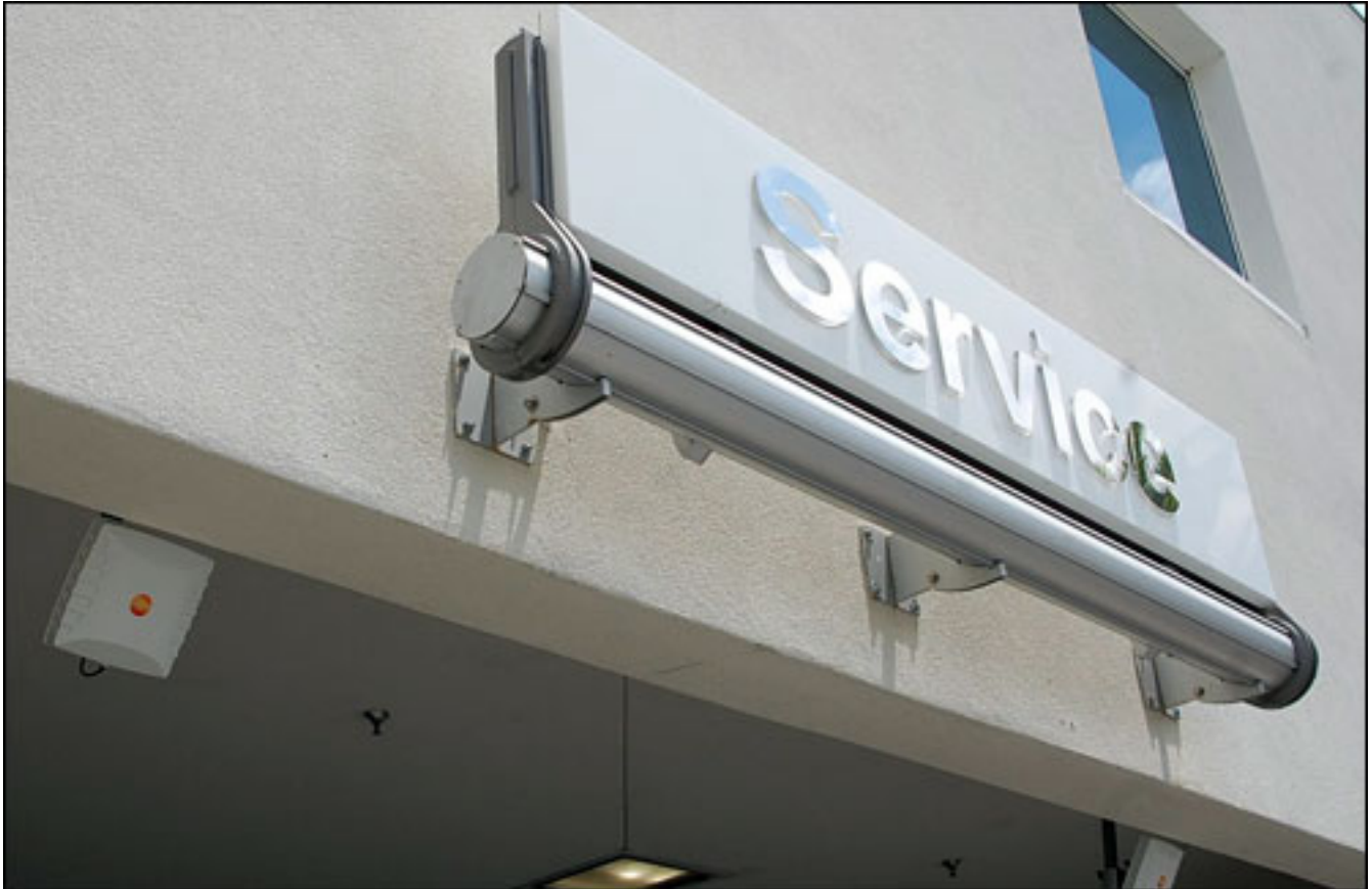
At the entrance to Fields BMW Winter Park's service area, a pair of RFID reader antennas identify a car's owner's upon arrival.
